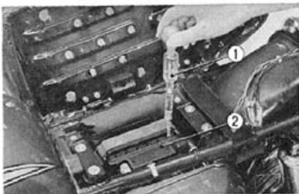
Fig. 19-15 ① Hydrometer ② Battery
