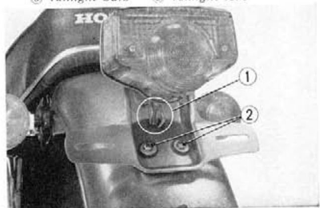
Fig. 16-7 ① Lead connectors ② Taillight bracket screws
