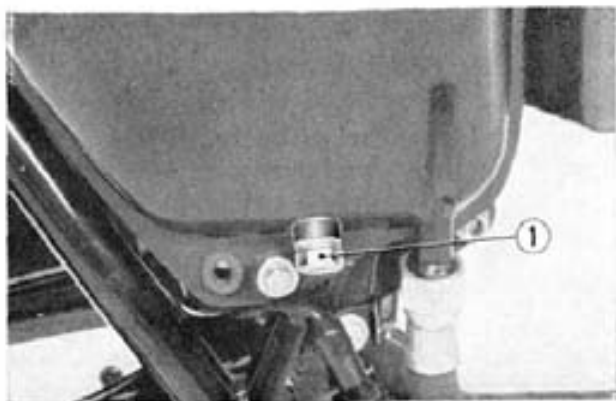
Fig. 19-1 ① Oil tank drain plug
